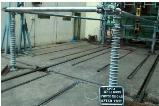
Figure 9: Post short circuit testing of 132 kV post.
