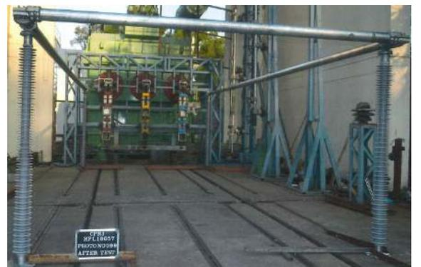
Figure 12: Post short circuit testing of 220 kV post
