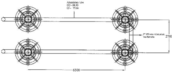
Figure 7: Testing schematic of 132 kV post insulators
