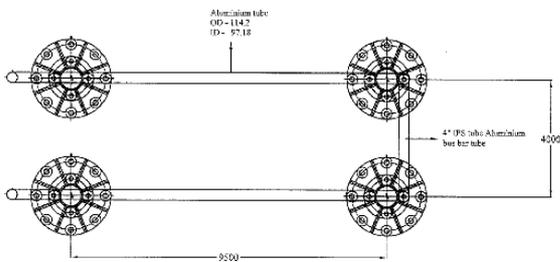
Figure 10: Testing schematic of 220 kV post.
