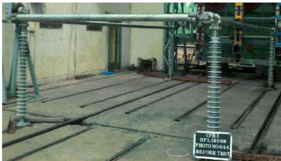
Figure 8: Pictorial testing arrangement of 132 kV post before short circuit test
