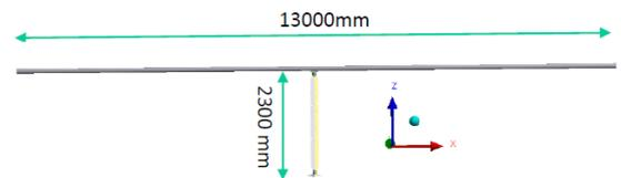
Figure 5: 220 kV post insulator modelled with a conductor of length 13m on top
