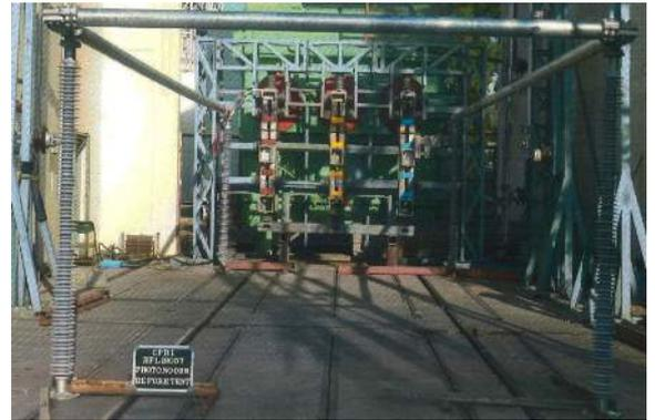
Figure 11: Testing arrangement of 220 kV post before short circuit test
