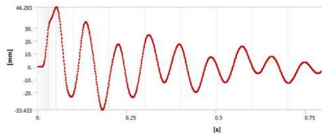
Figure 4: Simulation results of subjecting 132 kV post insulator for CIGRE model dynamic loading
