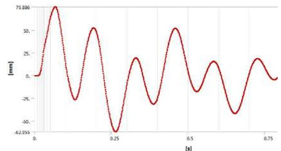
Figure 6: Simulation results of subjecting 220 kV post insulator for CIGRE model dynamic loading
